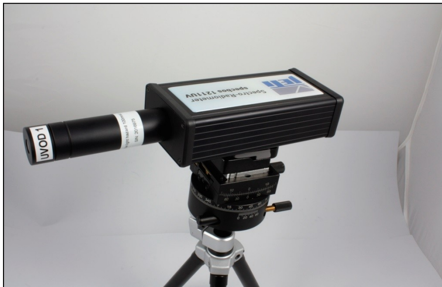
Fig. 8 Scheme of radiance based measurements (picture: specbos 2501-UV with 100 mrad optics and additional OD1 filter)
