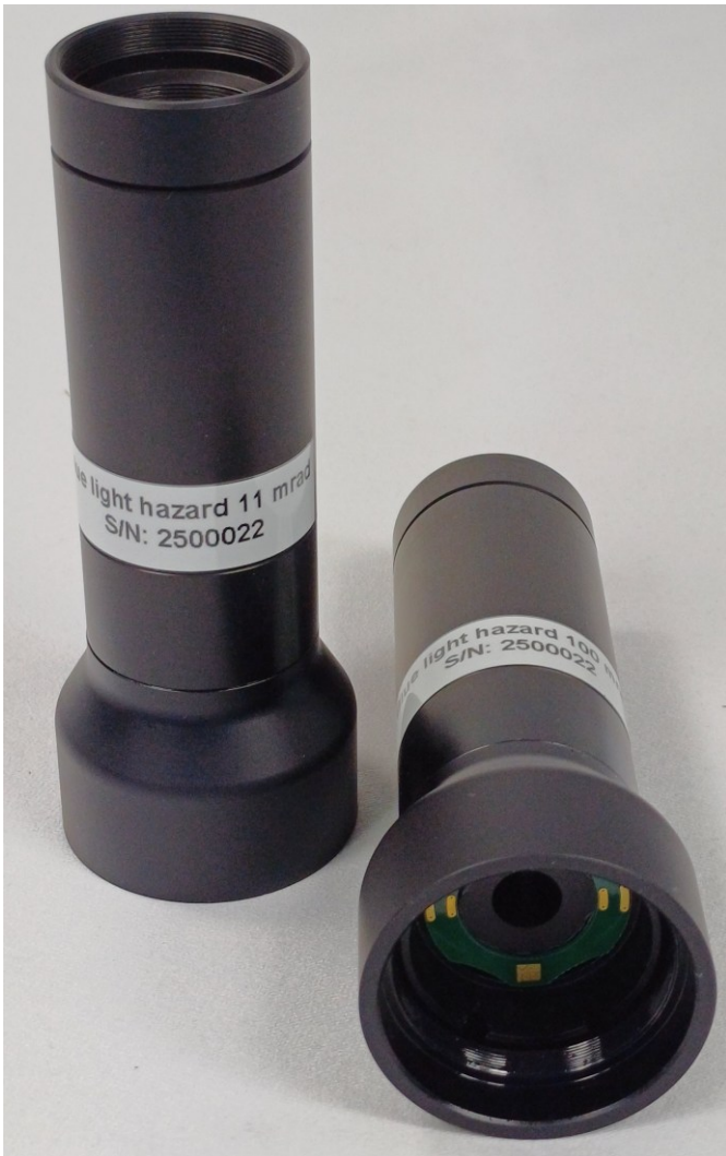
Fig. 2 Beam shaping optics for 100 mrad (ACC 080/100) and 11 mrad (ACC 080/11)
