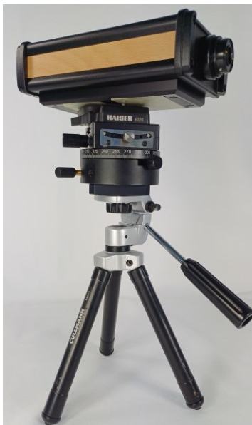
Fig. 5 specbos 2501-UV mounted on mechanical elements for turning/ tilting (ACC 025)
