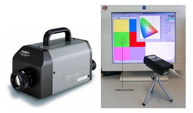
Fig. 6 Laboratory (CS-1000 of Minolta) and compact (specbos 1200 of JETI) spectroradiometer
