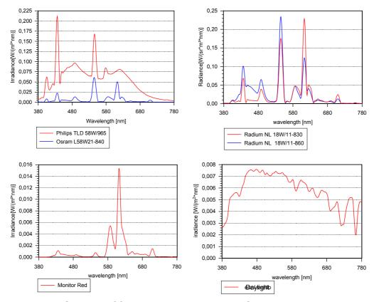
Fig. 2 Spectra of fluorescent lamps, a red CRT screen and daylight
