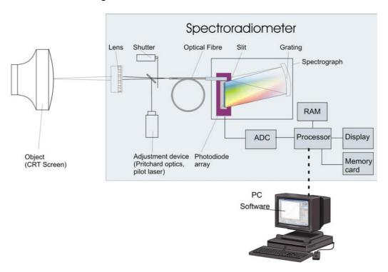
Fig. 3 Scheme of a spectroradiometer
