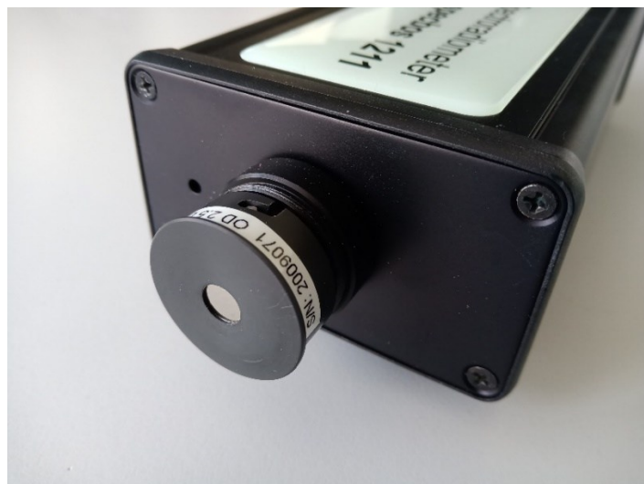
spechbos 1211-2 with attenuation filter cap
