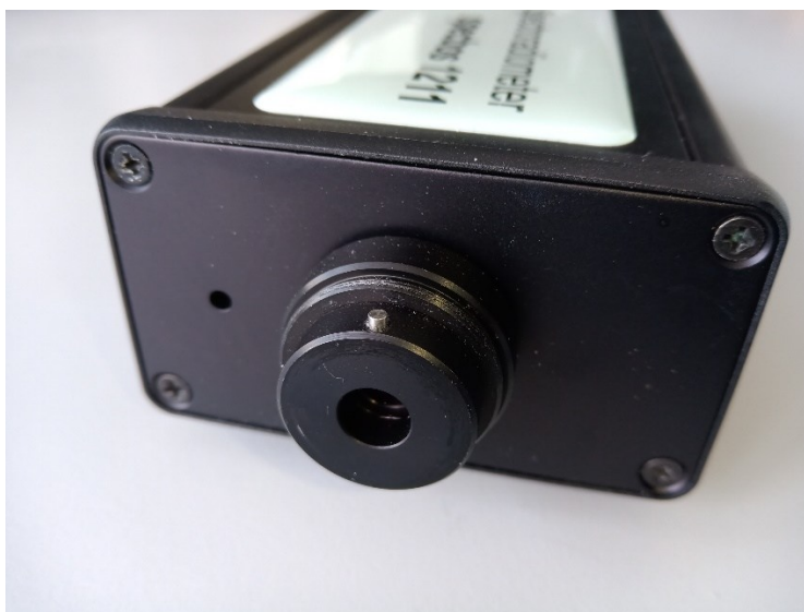
Front face of specbos 1211-2 with hole for sync detector (left of the measuring head)
