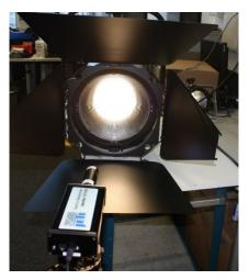
**specbos 1211UV-2** can be equipped with accessories for measurements of all photobiological measurements in the wavelength range of 230 ... 1000 nm, defined by EN 62471.
