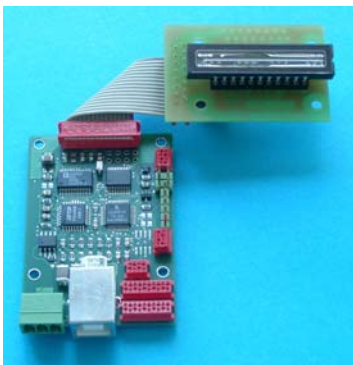
Fig. 18 Universal controlling electronics VersaSpec for different photodiode and CCD detector arrays (example Sony ILX571)
