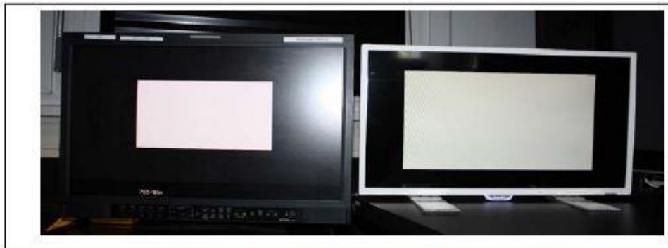
Figure 9. Experiment 2 with two different LCD monitors (left: CCFL backlight, right: LED backlight)
