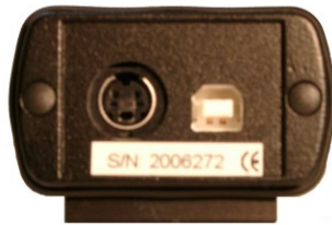
Figure 1: Backside of specbos xx01 (right – USB, left – trigger)
