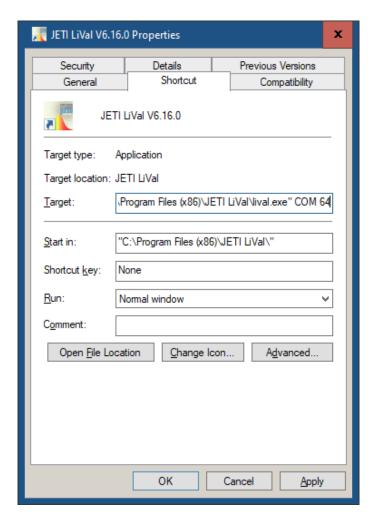
Type the number of the COM port to be used after the filename of the executable in the 'Target' box (COM 4 for COM4 in this example). Use a space sign between the filename, the tag COM and the port number.
