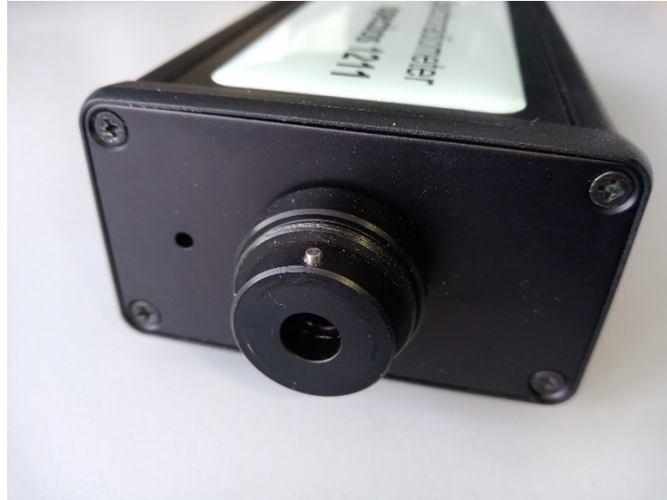
Front face of specbos 1211-2 with hole for sync detector (left off the measuring head)
